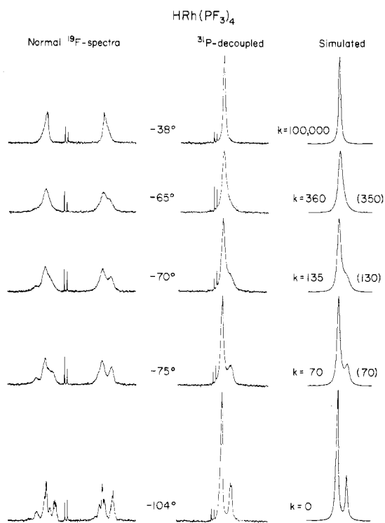
Figure 2. Normal and 31 P-noise-decoupled 19 F NMR spectra at 56.45 MHz of HRh(PF 3 ) 4 in CHF 2 Cl at various temperatures with calculated NMR line shapes at rates ( K ) indicated.
